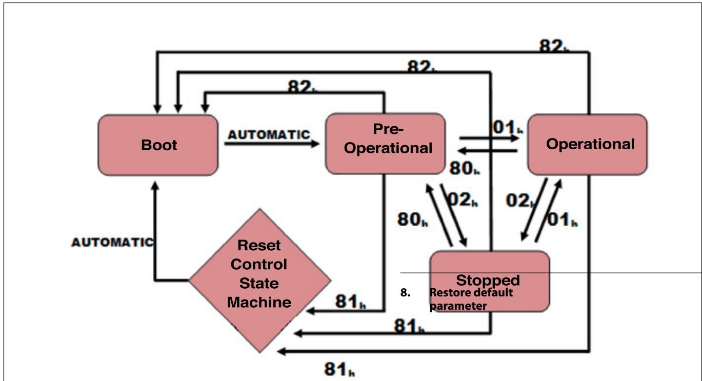
Every CANopen device contains an international Network Management server that communicates with an external NMT master. One device in a network, generally the host, may act as the NMT master. Through NMT messages, each CANopen device's network management server controls state changes within its built-in **Communication State Machine**. This is independent from each node's operational state machine, which is device dependant and described in **Control State Machine**.
